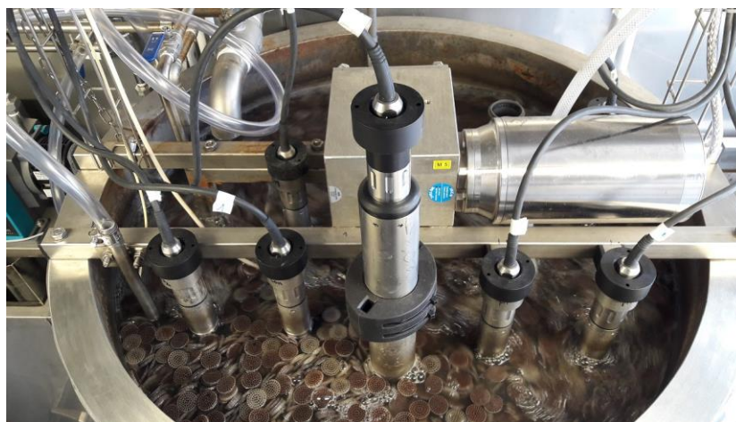
Fig. 3 View of the HMBBR reactor equipped with in-line instruments
